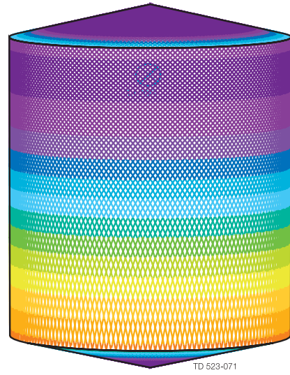
D4.6m H5.5m, Toftejorg MultiJet 25, 4 x ø5.5 mm Time = 8.3 min., Water consumption = 1612 l (426 gallon)
