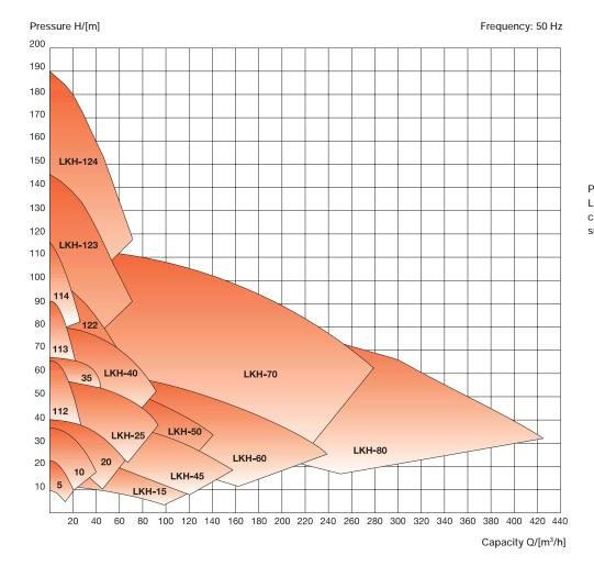
Performance across the range. LKH series pumps are available with capacities up to 440 m<sup>3</sup>/h and pressures up to 190 m (19 bar/275 Psi).
